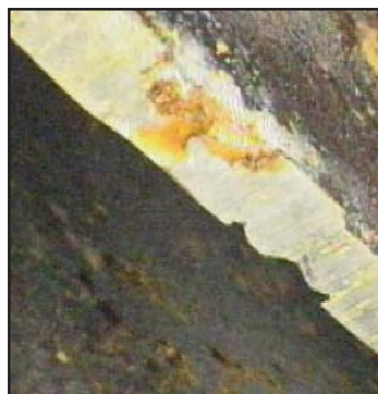
Rotor blades - worn and new - as viewed by a fiberscope
